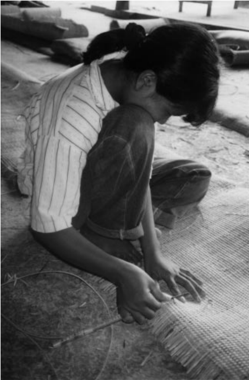
Finishing the irregular patches in rattan webbing, Rengasdengklok, West Java, Indonesia (Photo: Rita Mustikasari)
