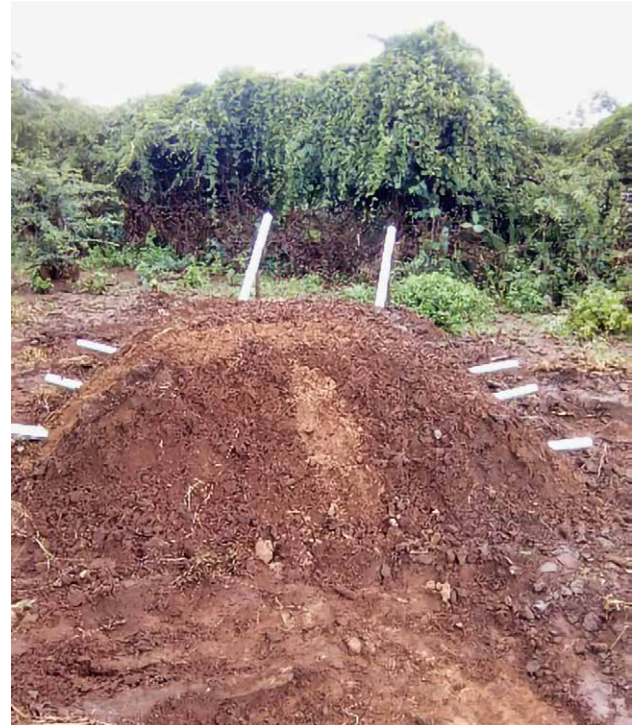
Figure 10. Improved earth mound kiln.
