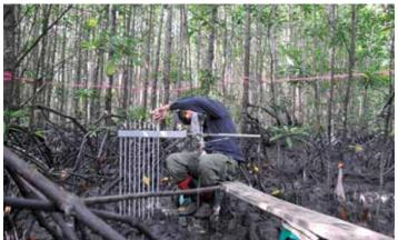
The use of rod surface elevation table (rSET) combined with marker horizon to estimate surface elevation change and sediment accretion rate (Photo by Sofyan Kurnianto/CIFOR)
