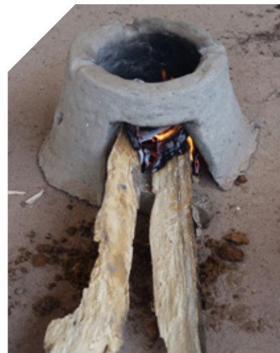
Prototype of improved cookstove made with locally available materials
