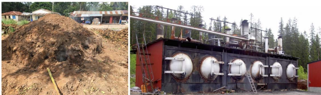
Figure 2. Traditional earth mould kiln in Tanzania (left) and Silos kiln from which gaseous energy is used for district heating at Umeå, Sweden (right). Photos: Mary Njenga/ICRAF (left) and Hakan Örberg (right).
