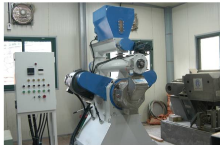
Fig. 1. Image of ring-die type pelletizer used for the pellet production in this study.
