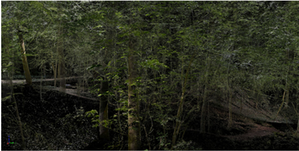
Fig. 1. Point cloud of Wytham Woods generated from a TLS campaign where 176 scan positions were co-registered. Concurrent RGB images were captured with each scan, the images and point cloud were then co-registered and points are attributed with an RGB value. An animated fly-through of this scene can be viewed at https://www.youtube.com/watch?v=RS6q3HMEJK8 .
