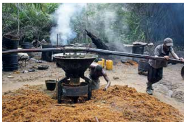
Figure 11. Milling of boiled fruits to produce crude palm oil.
