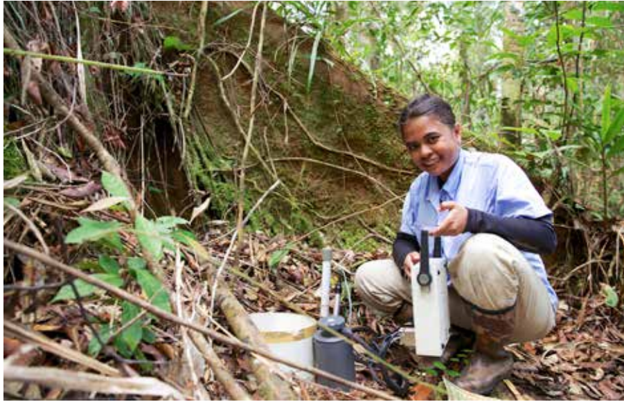
Figure 25. The measurement of CO 2 using a dynamic chamber method with portable infrared gas analyzer.
