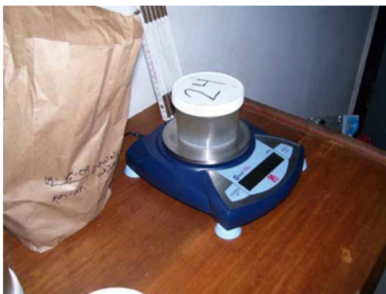
Figure 21. After drying samples to a constant weight in a drying oven at temperatures \leq 60 °C, samples are then weighed with a digital balance. As the sample consists of a known field volume, the bulk density can now be determined.
