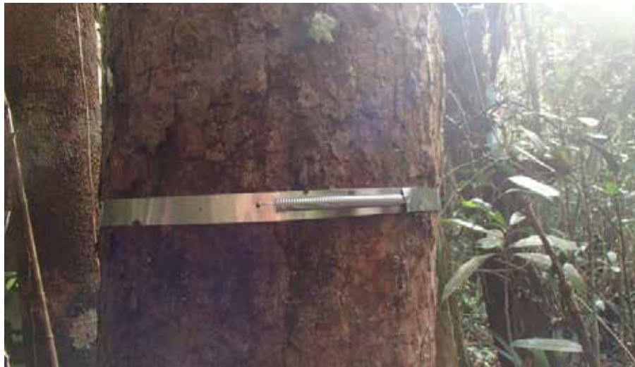
Figure 27. A dendrometer band for measuring the tree diameter growth.
