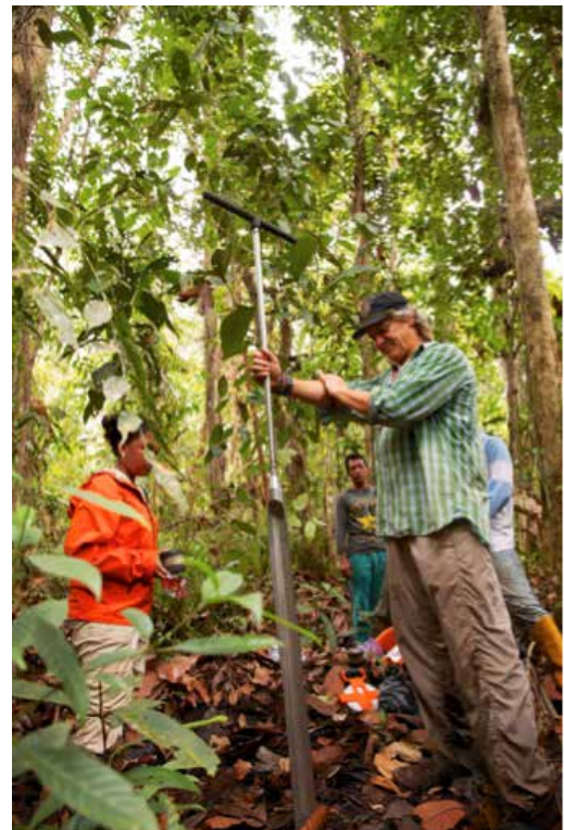
Figure 17. An open-faced auger is quite efficient for sampling in shallow peats.
