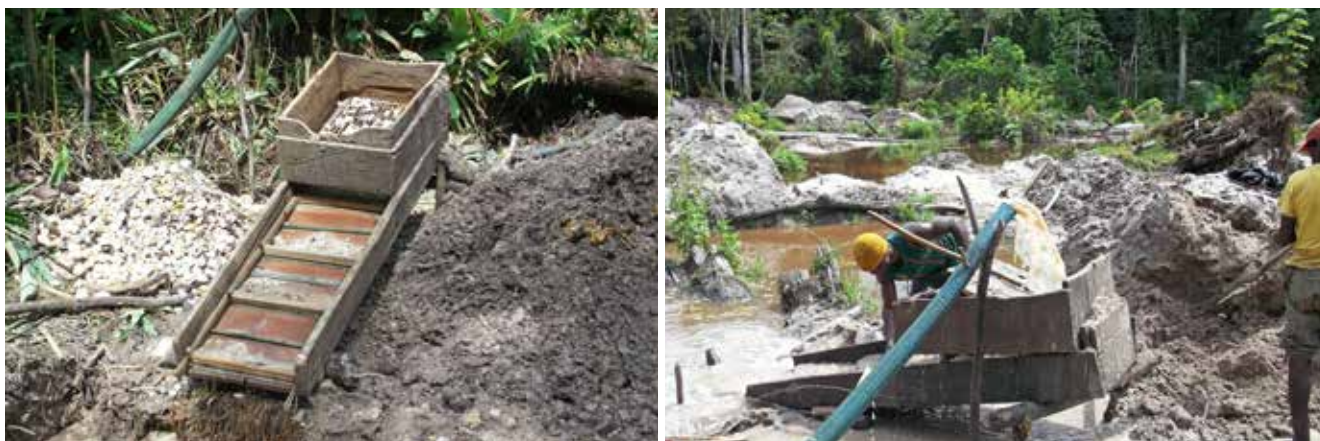
Photo 1. A wooden sluice box and gold washing process in NMFM.
