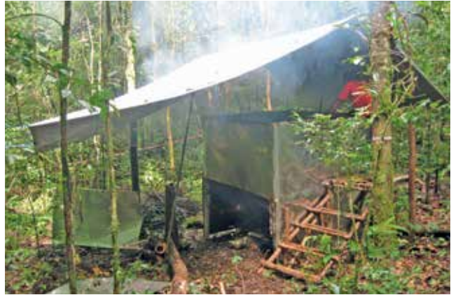
Figure 2. One of the field ovens used to dry the subsamples on location.
