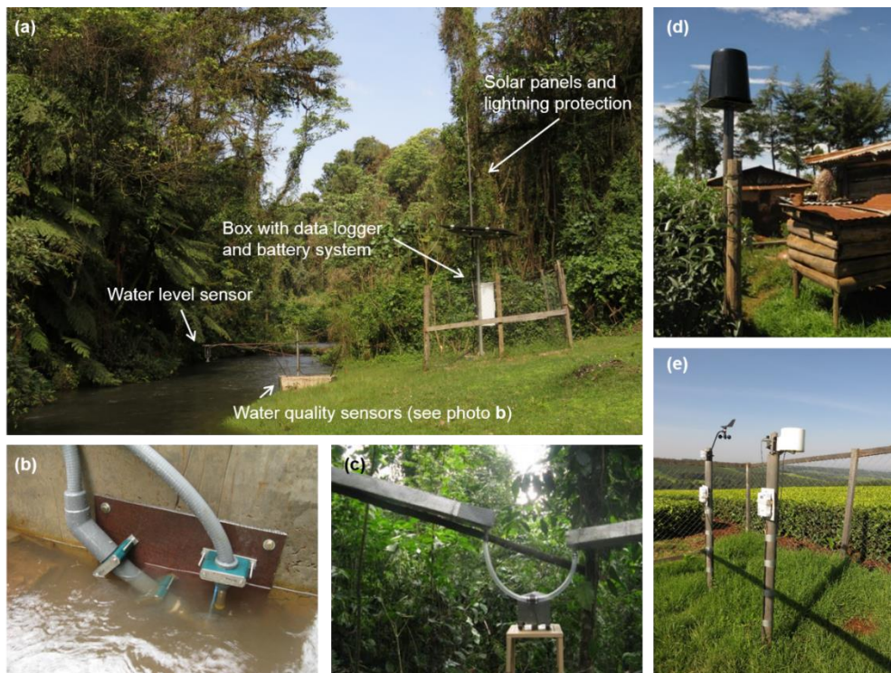
Figure 2 Instrumentation in the study catchments: (a) automatic measurement system for water quality and quantity, (b) water quality sensors with spectrometer (left) and electrical conductivity probe (right), (c) throughfall tipping bucket, (d) tipping bucket and (e) weather station.
