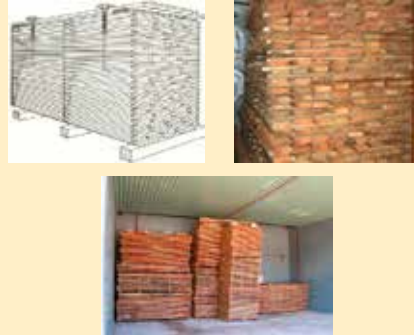
FIGURE 2. Stacking technique of wood in the drying chamber
