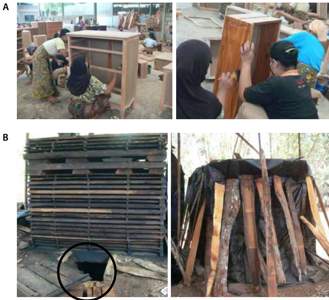
Figure 1. Brushing method on furniture component (A) and smoking method on sawn timber (B)
