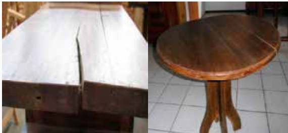
Figure 4. End checking of timber and warping of furniture
