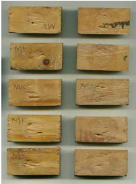
Figure 2. Drywood termite attacked samples
