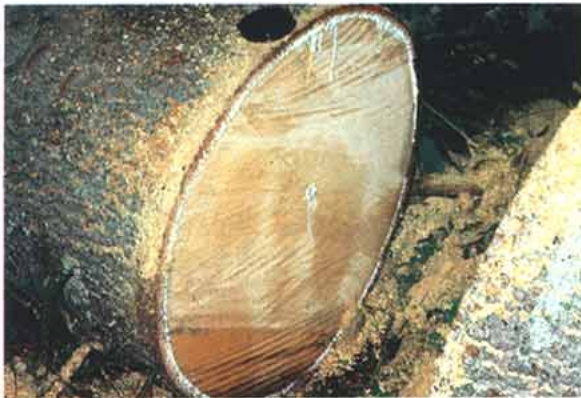
Figures 5b and 5c. Transverse (b) and radial (c) surfaces of freshly-felled jelutong ( Dyera costulata ) with latex oozing from the bark, pith, and rays. The Rubber Research Institute of Malaysia has found that latex is a suspension of latex chemicals, mitochondria, ribosomes, and other sub-cellular organelles.
