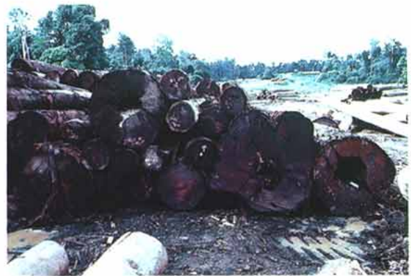
Figure 5e. Logs of chengal ( Neobalanocarpus heimii ). The large logs are hollow while the small logs are solid, indicating is that large logs are much older than 100 years, which is the known limit of durability of chengal timber in usage under exposed conditions.
