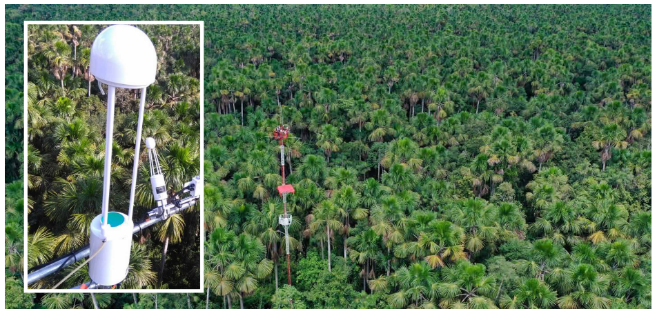
Eddy covariance tower for intensive carbon monitoring over palm ( Maruritia flexuosa ) dominated peatlands, Quistococha, Iquitos, Peru. Photo: Lizardo Fachín/IIAP
