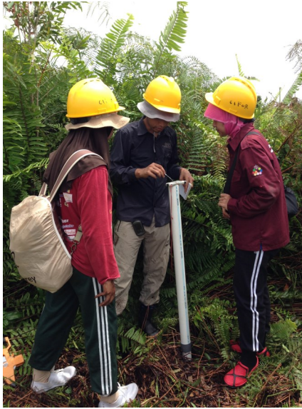
IPN internship students installed water table monitoring station in degraded peatlands in Central Kalimantan (Photo by Daniel Murdiyasar/CIFOR)
