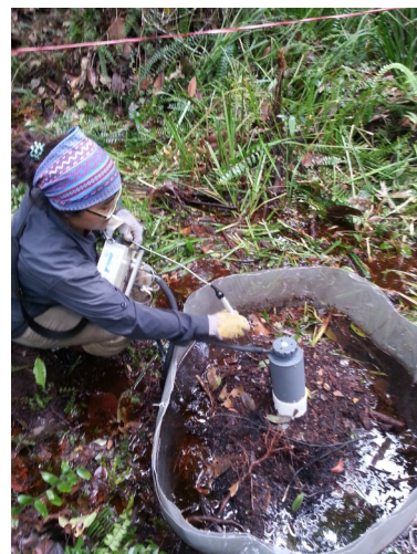
IPN internship student measured heterotrophic respiration in forested peatlands by using portable gas analyzer (Photo by Kemen Austin/CIFOR)
