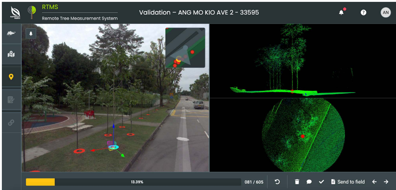
Photo 2. The Singapore National Park Board's Remote Tree Management System (RTMS) uses a combination of LIDAR, drones, digital twins and geospatial mapping to remotely assess the health of and management options for all 6 million trees under the Board's manage (© National Park Board).
