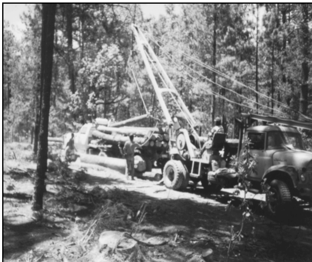
Figure 1. Motogrúa used for timber yarding and loading.
