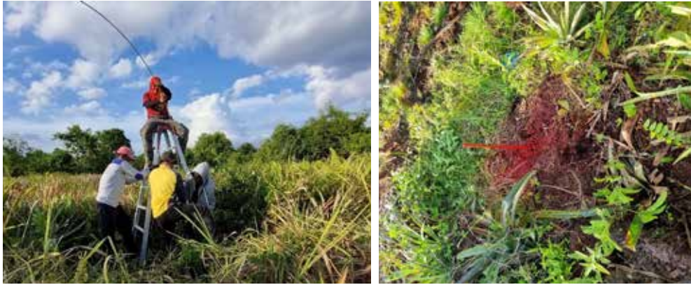
Figure 13. Installing subsidence poles
