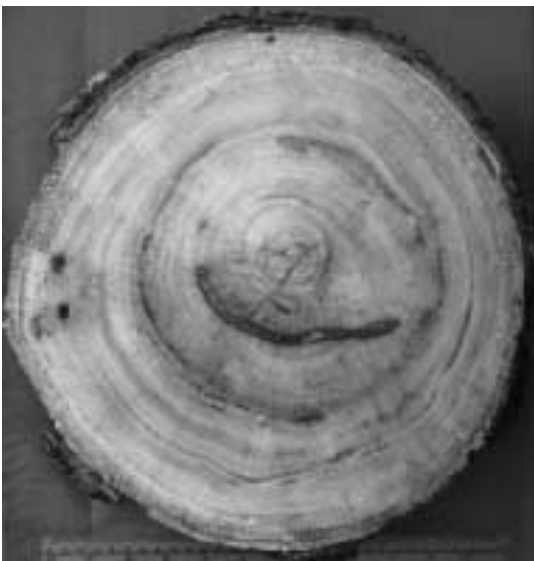
Photo 14. Fungi attacking only sapwood and followed by insect borers in heartwood of medang ( Litsea sp.) (Type II)
