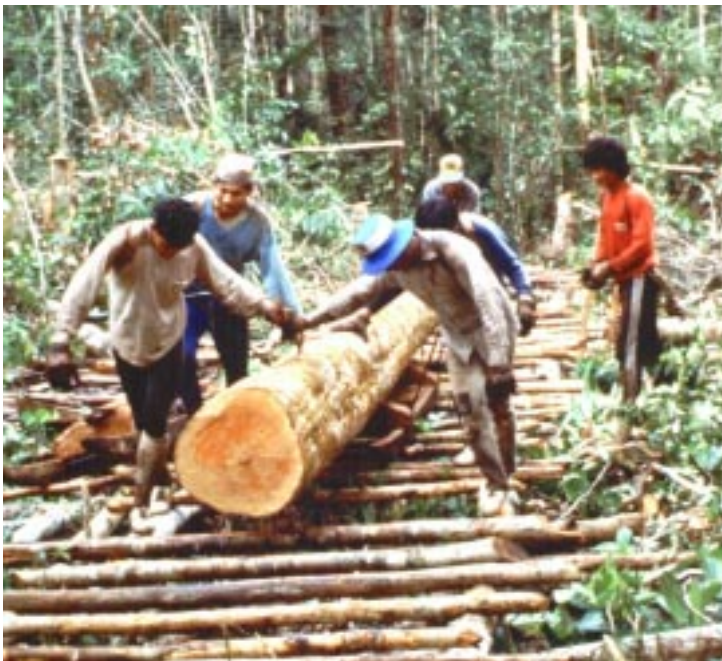
Innovative adaptation of skidding for logs on swampy soils (photo by John Turnbull).
