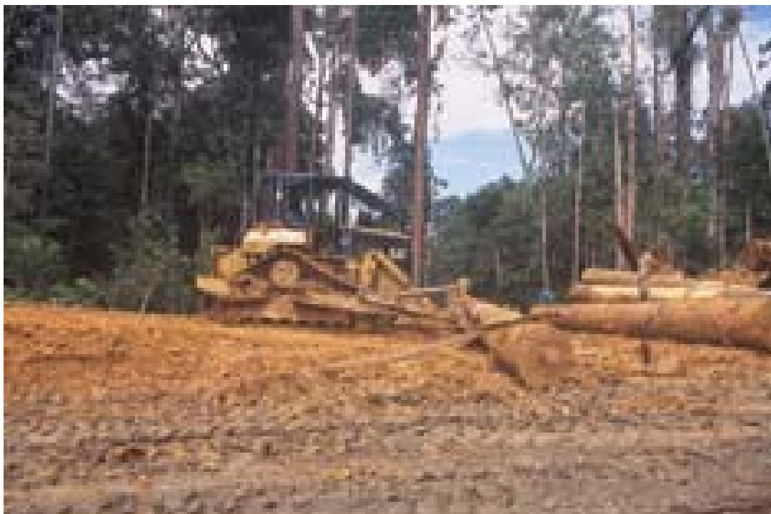
CAT 527 Skidder and log landing in RIL operation
