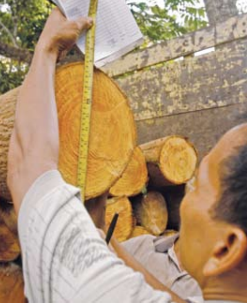
A log trader measures the diameter of a log to determine its quality and selling price
