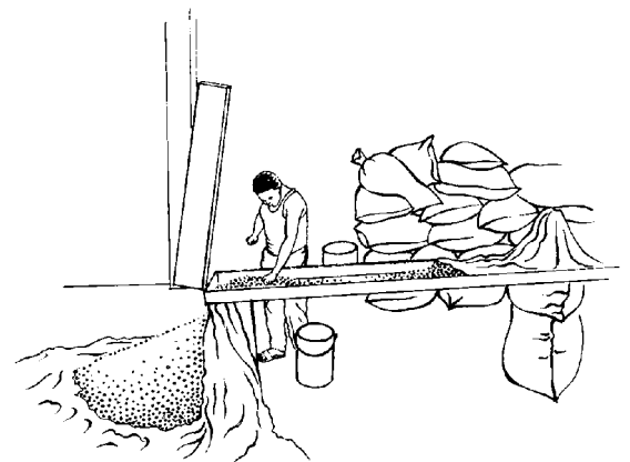
Grain sieves are used to assist the sorting process - helping to weed out damaged berries and separate the rest according to size.
