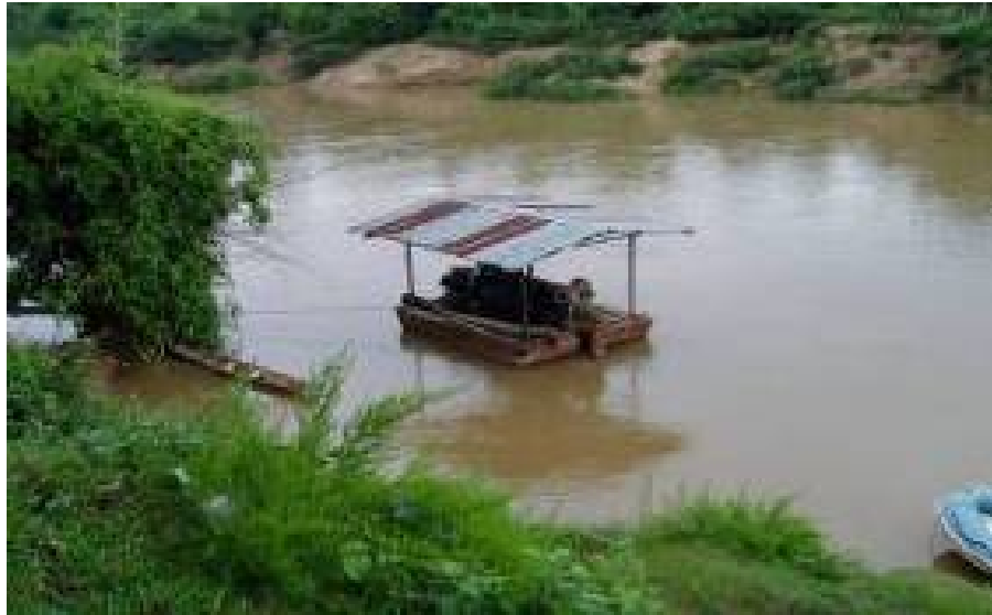
Plate 4: Dry season diesel irrigation boat and pumps, upstream at Ban Pak Theuk.
