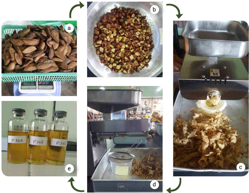
Figure 2. Pongamia oil extraction process using a mechanical press: (a) pongamia pods/fruits, (b) dry pongamia seeds, (c) pressing process, (d) filtering process, (e) pongamia oil
