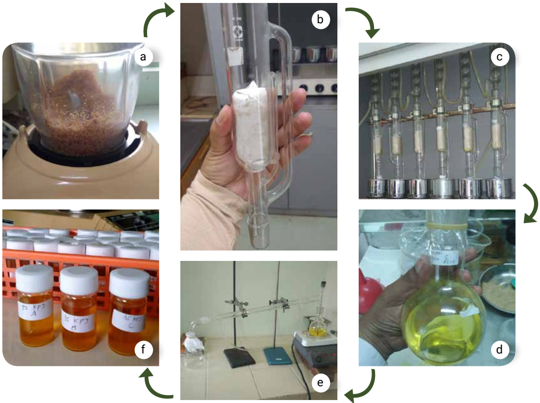
Figure 3. Pongamia oil extraction process using the solvent method: (a) seed grinding, (b) thimble in chamber, (c) oil extraction process by Soxhlet extractor, (d) raw oil and n-hexane solution, (e) distillation process, (f) pongamia oil
