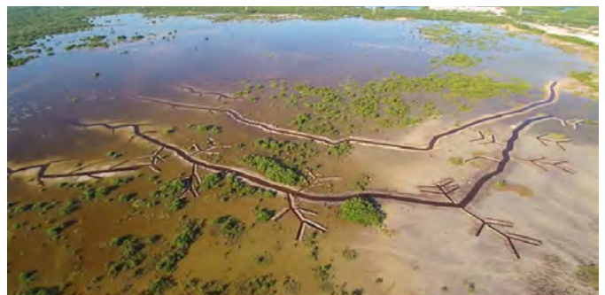
Rehabilitated channels with zig-zag pattern. Progreso, Yucatán.
