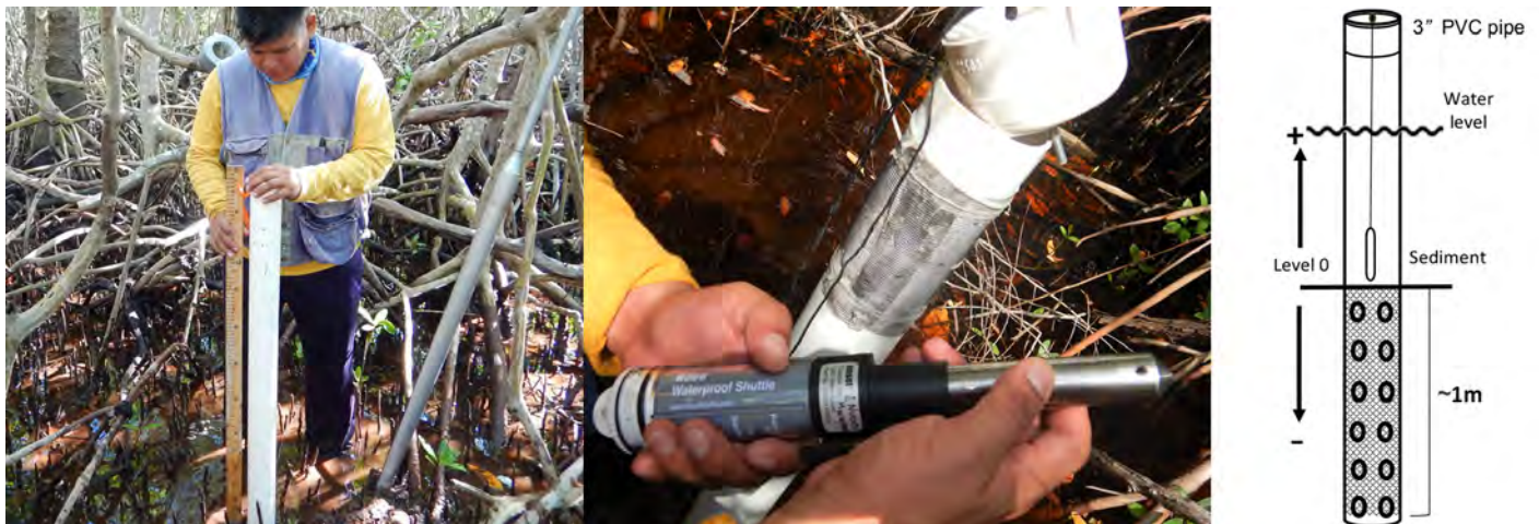
Figure 9. Installation of automatic pressure sensors at the reference and degraded sites.
