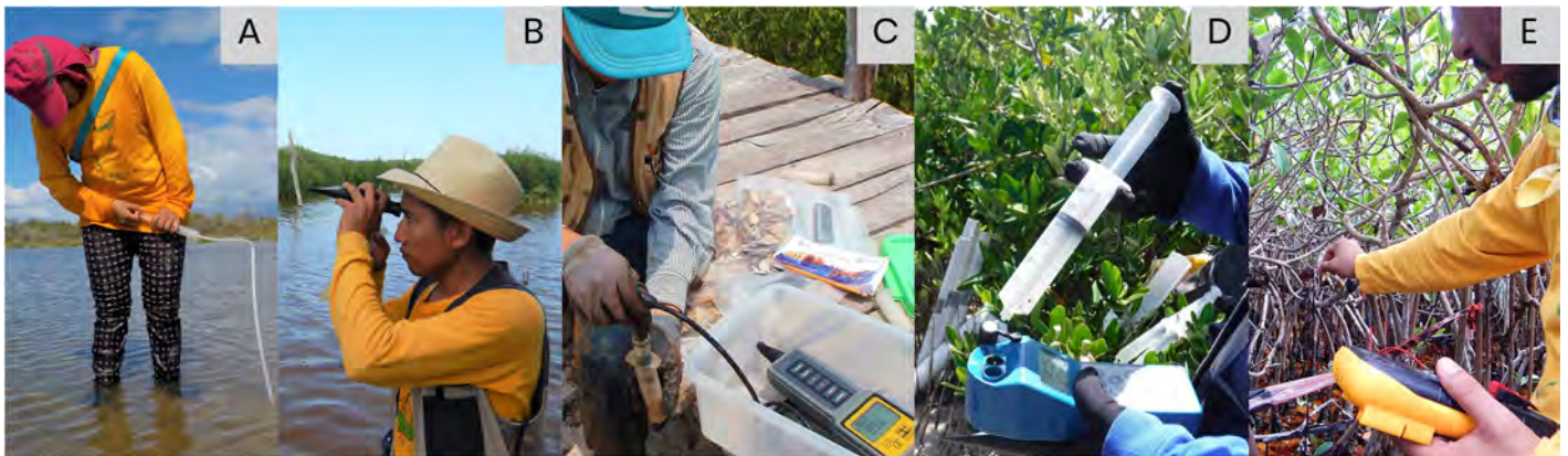
Measuring physical-chemical characteristics of water. A) Collecting a sample of interstitial water. Measuring interstitial salinity with B) refractometer and C) multiparametric probe. D) Measuring redox potential and pH with a field pH-meter, and E) measuring redox potential with copper rods, a voltmeter and a platinum electrode.
