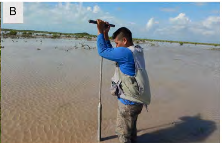
Collecting sediment cores with A) PVC tube, and B) metal tube.
