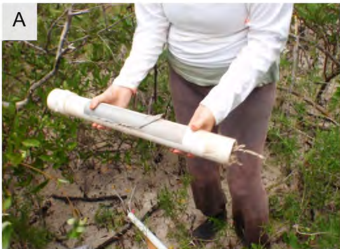
Collecting sediment cores with A) PVC tube, and B) metal tube.
