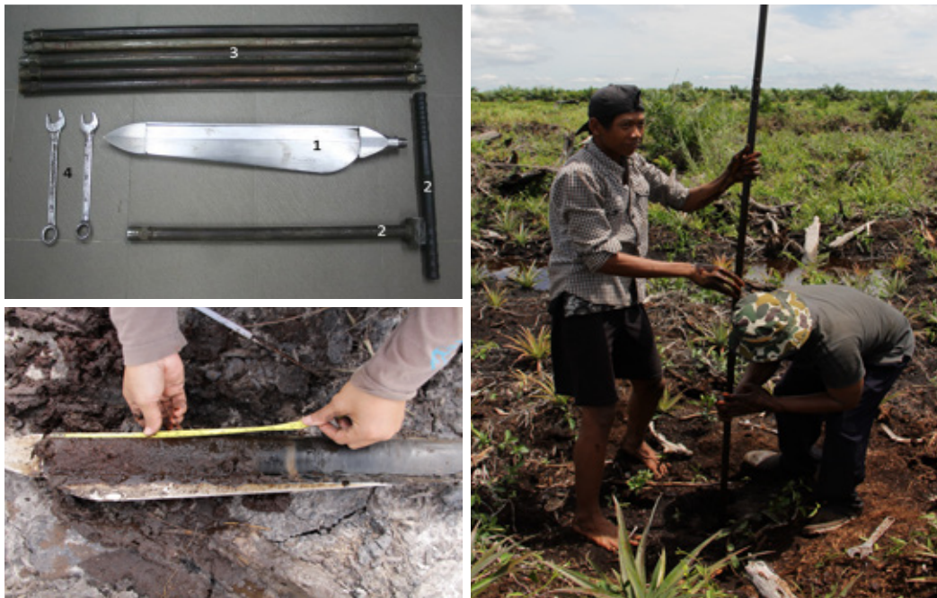
Figure 4. Peat sampling using peat auger
