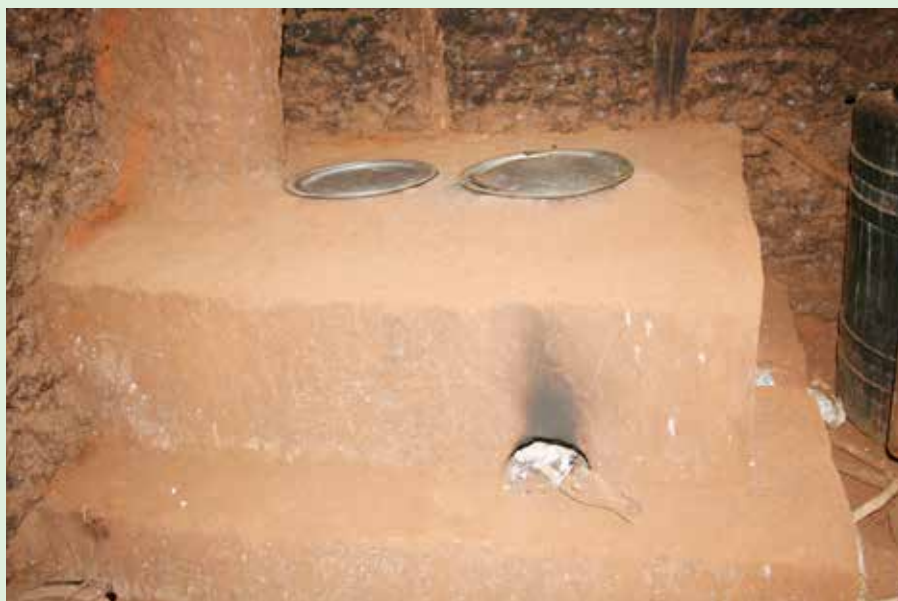
Improved cooking stoves exist in various forms. This one, as photographed from a household in Tharaka-Nithi, economizes on the use of firewood, and has a chimney to guide all smoke outside of the kitchen. Photo BGF.
