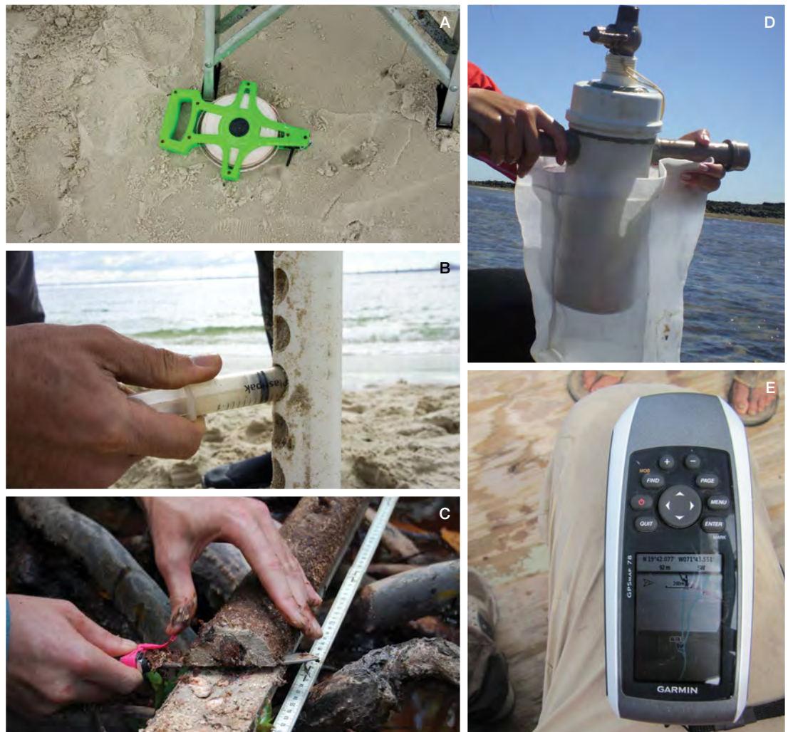
Figure 3.3 Equipment typically needed for field collections of soil carbon. (A) Measuring tape for measuring depth along the soil core (© Sarah Hoyt, CI), (B) Syringe used to subsample core (© Sarah Hoyt, CI), (C) Knife used for subsampling (© Boone Kauffman, OSU), (D) Core & sample bag (© Margareth Copertino, FURG), and (E) GPS to mark coring position (© Boone Kauffman, OSU)
