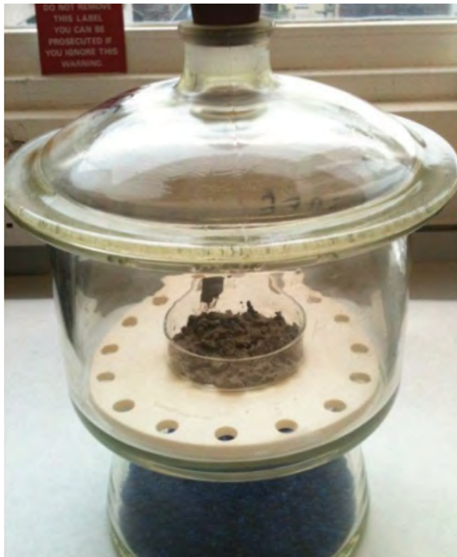
Figure 3.18 Soil sample cooling to room temperature in desiccator (© Hilary Kennedy, UWB)
