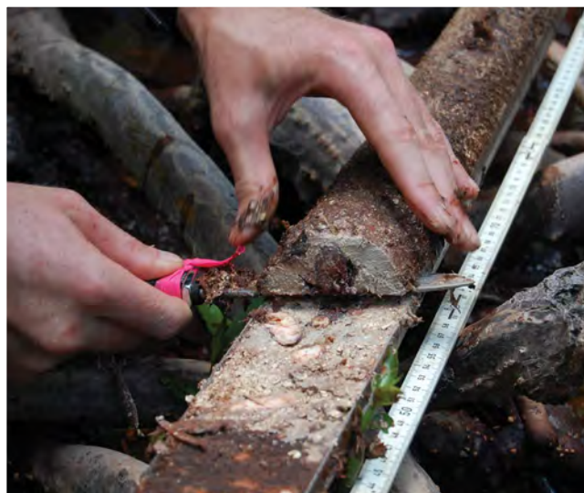
Figure 3.10 Soil core liner that has been cut lengthwise to expose the soil for archiving and subsampling. This core is in the process of being split. A clean face is exposed in the lower part of the image. (© Boone Kauffman, OSU)
