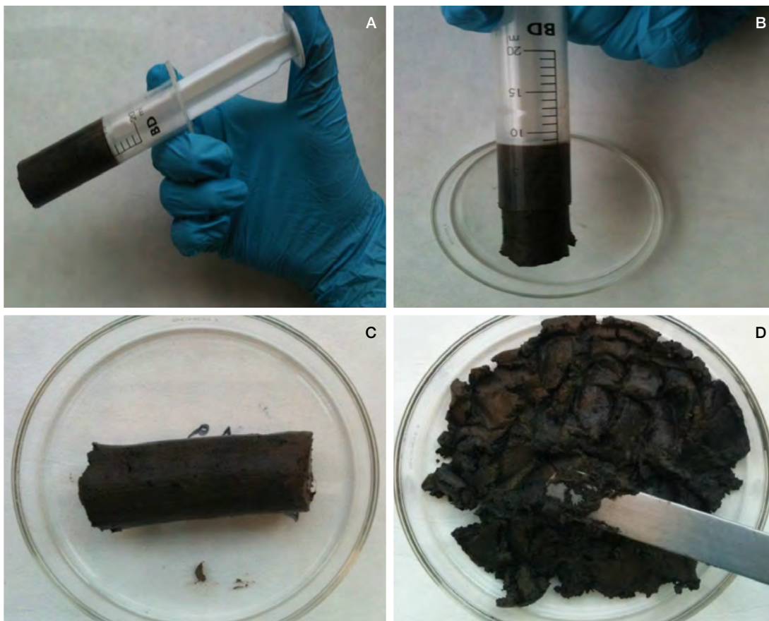
Figure 3.17 Removal of sample from syringe and preparing it for oven drying. (A) Sample in syringe, (B) Depositing sample on pre-weighed petri dish, (C) Sample when first removed from the syringe, and (D) Spreading the sample with a spatula. (© Hilary Kennedy, UWB)
