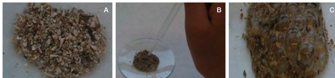
Figure 3.24 Testing for carbonate. (A) Subsample in a watch glass prior to acidification, (B) pipetting a few drops of weak HCl, (C) subsample effervescing. (© Hilary Kennedy, UWB)
